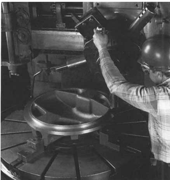
Cast domed disc being machined.
